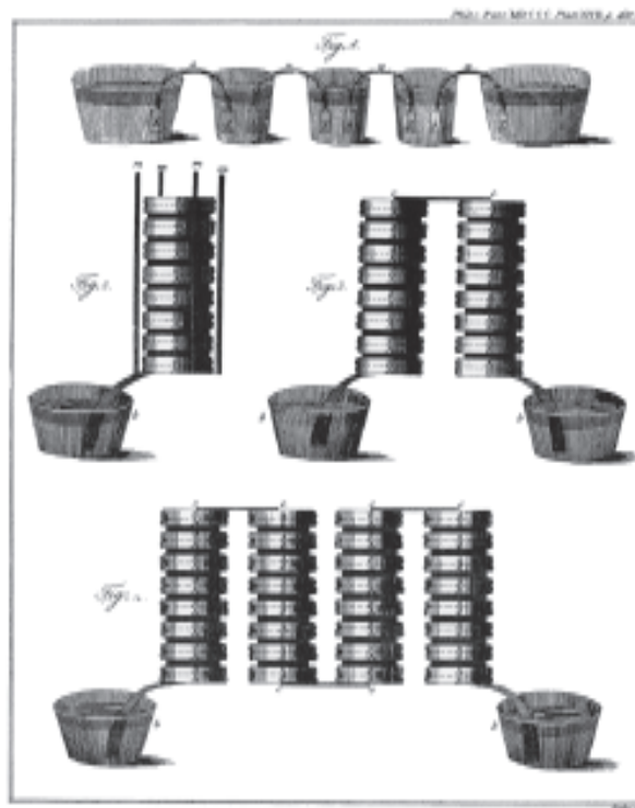
Figure 3. Four connections of "voltaic piles" (alternate silver and zinc discs separated by moist paper) as described in A. Volta's letter to Sir Joseph Banks of the Royal Society of London bearing the title, "On the Electricity excited by the mere Contact of conducting Substances of different kinds," dated March 20, 1800.
